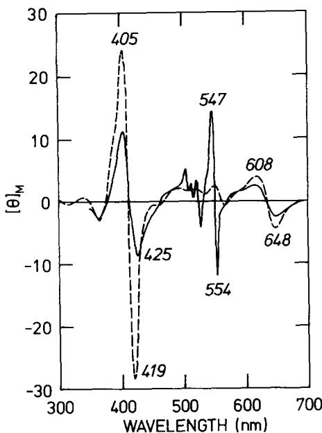
Fig. 1. MCD spectra of *Pseudomonas* nitrite reductase. Ps.NiR(4.47  $\mu$ M) was dissolved in 0.1 M Tris-HCl, pH 7.93. -----, oxidized form; —, reduced with sodium dithionite.  $[\theta]_M$  is molar ellipticity per unit magnetic field strength.
